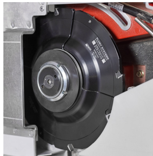
Adjustable grooving tool with reversible carbide tips
